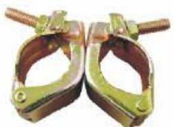
110° Pressed Swivel Coupler 48.6mm/0.58-0.65kg
